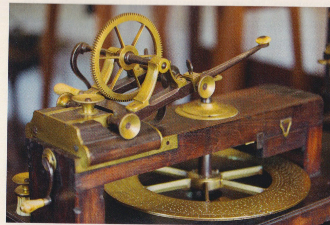
Figure 3. Eighteenth-century wheel-cutting engine. Courtesy of Willard House and Clock Museum.
