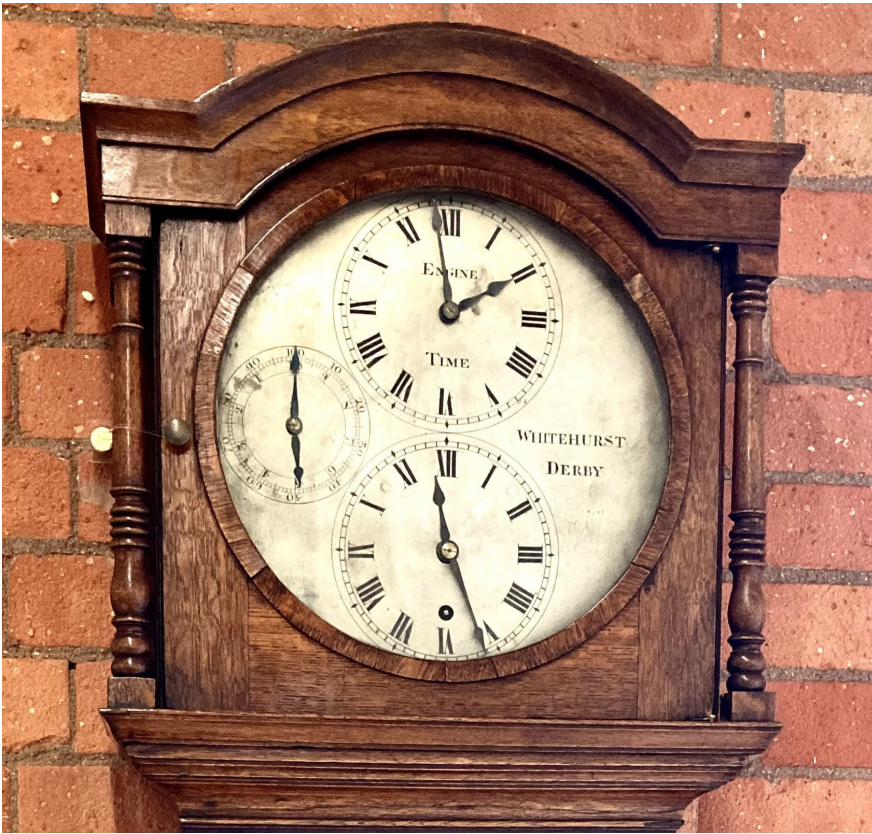
Fig. 8. Whitehurst mill clock, c.1811, Museum of Making, Derby. Photo by the author. The upper dial marked 'ENGINE TIME' indicates the weekly hours when factory machines were running. The dial on the left, marked 0-100, and on the inner ring 0-10 counterclockwise, is believed to show revolutions of the engine.
