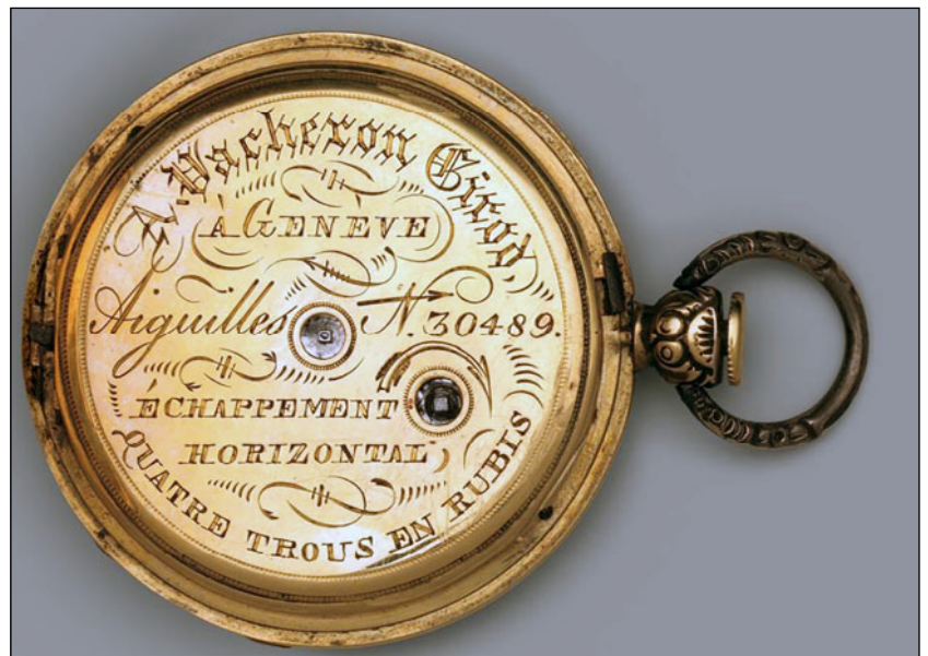
Figure 4. The rear cover of this 1832 pocket watch by Abraham Vacheron Girod provides details about what is inside. Many nineteenth-century Swiss watches had similar engraved information noting, as this does, the tiny drilled jewels used as low-friction bearings. The Swiss firm Vacheron & Constantin still produces fine watches.
