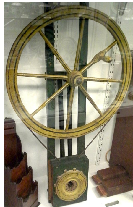
In the "attic" visible storage of Historic Deerfield's Flynt Center is an example of Rufus Porter's corn sheller, patented in 1838. To operate, the farmer used one hand to turn the large wheel, while the other hand fed ears of corn into the aperture below. We have no reports on how well this worked. Frishman photo.
