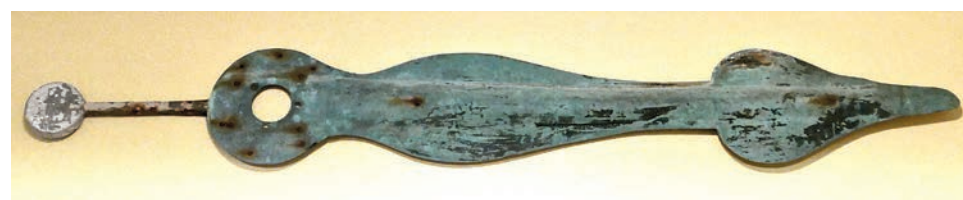
Figure 16: Antique tower clock hour hand. Note counterweighted tail to perfectly balance hand at its center hub. Author's collection.
