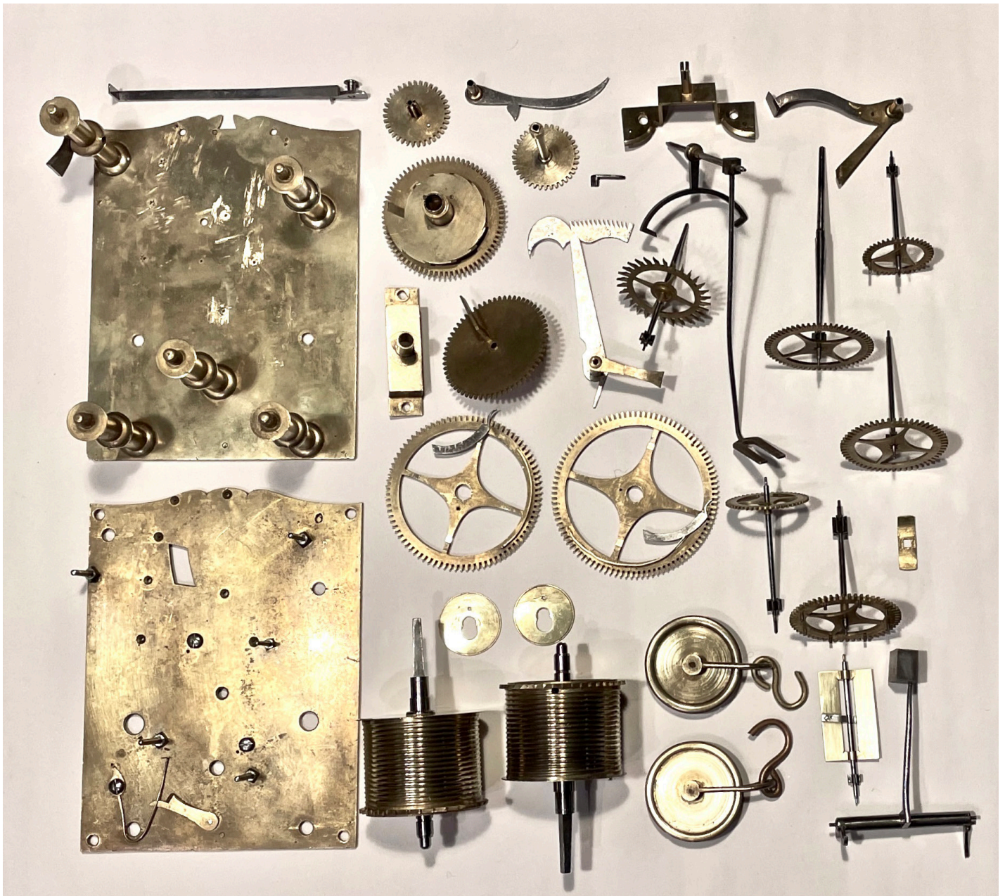
Fig. 1. Disassembled brass-and-steel movement of a Jonathan Mulliken tall clock.
