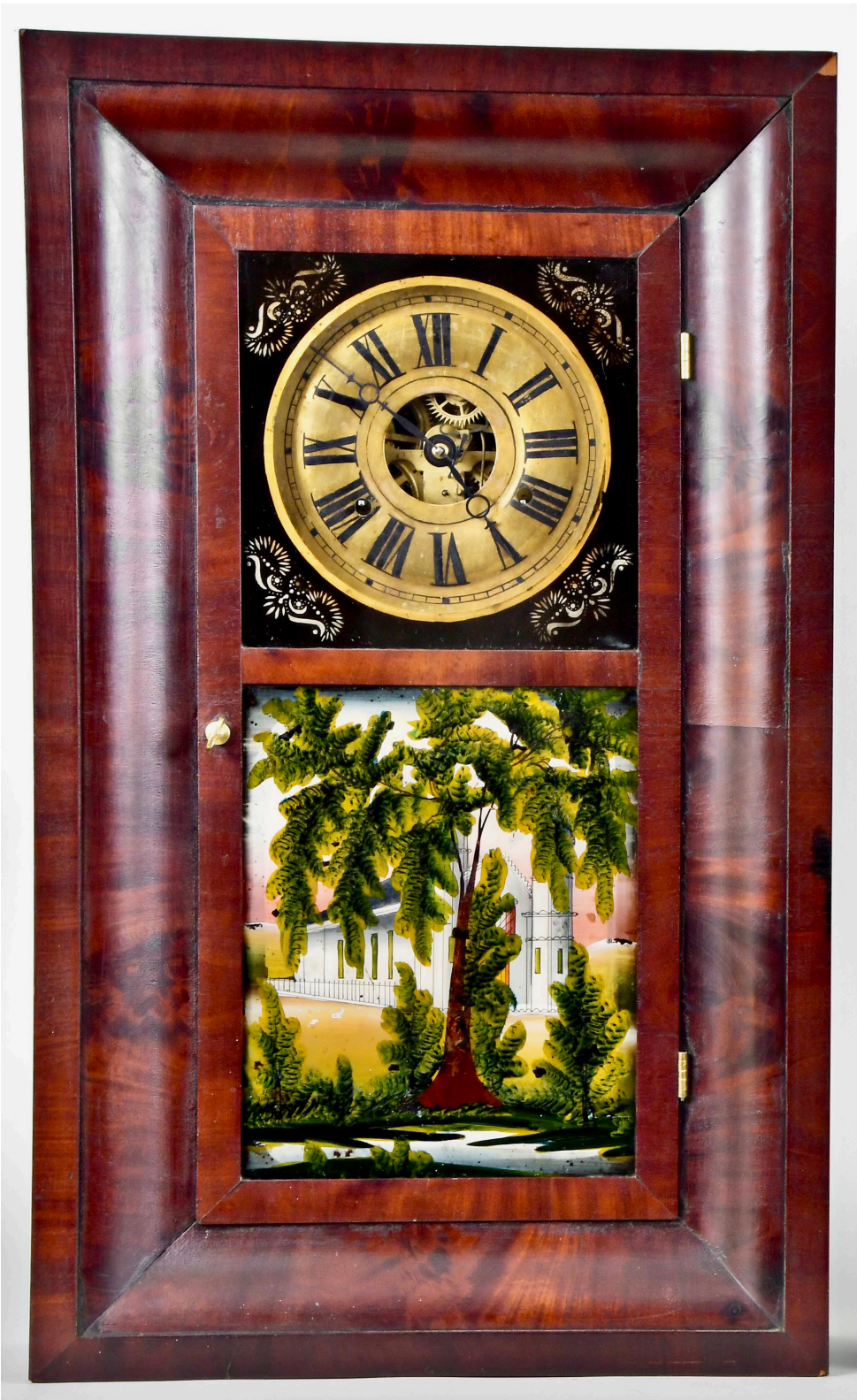
Figure 13. Chauncey Jerome "OG" shelf clock. Note the dial's large center opening which allowed a view of the brass movement, confirming at the time that it was not an obsolete wood movement.
