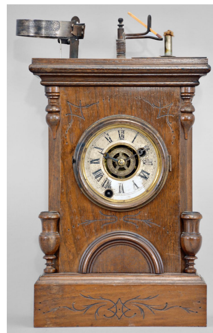
The Ansonia Brass & Copper Company in Connecticut produced this circa 1877 novelty alarm clock. At the selected time, a match would strike and light a small lamp, or if the owner was unlucky, the lit match would fly across the room and set the curtains ablaze. Artist and polymath inventor Rufus Porter (1792-1884) patented a similar concept clock back in 1833. This complete example, rarely found, sold for $1610 (est. $700/900).
