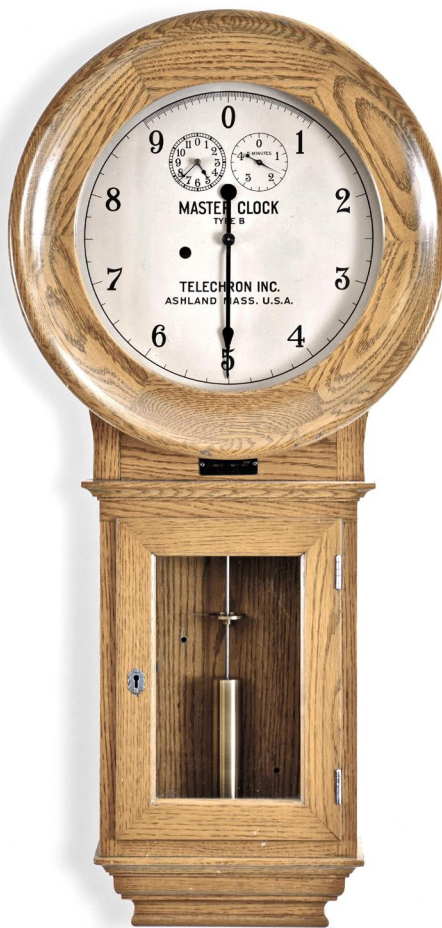
In order for the Warren Telechron Company, Ashland, Massachusetts, to sell its plug-in electric clocks in the 1920s, power stations needed to produce alternating current at precisely 60 cycles. Variations would greatly affect the accuracy of those clocks. Telechron made regulators for those power plants, allowing the operators to adjust the generator’s revolutions per minute and to adhere to the required frequency output. This oak model sold for $920 (est. $400/600).
