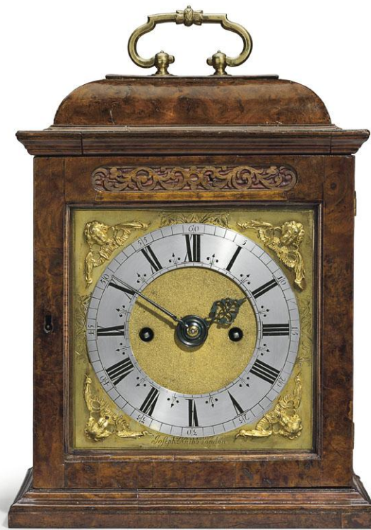
The English clocks in the sale were of uneven appeal, but this circa 1685 London table clock by Joseph Knibb exceeded, with premium, its high estimate when it sold for $221,000. The maker's prominence in English clockmaking history and the clock's unusual "double-six" striking contributed to the strong price. Designed to extend mainspring power, "double-six" counted the hours only from one to six, then started over. Most of us could figure out that six dings in the middle of the day or night actually signals twelve o'clock, but obviously the concept did not catch on.
