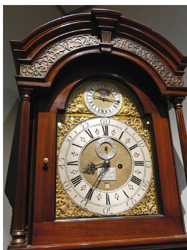
The tombstone dial of this circa 1748 clock by William Claggett displays additional complex functions in its top arch. The moon phase is revealed in a less common "penny moon" format. The silvered numbered rings indicate the date of the lunar month and the time of local high tides, information perhaps still useful to the clock's private owner.
