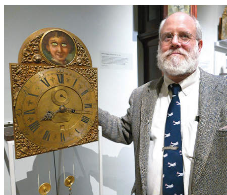
Massachusetts clockmaker Peter Nunes stands with the William Claggett movement he completely restored for the exhibit. The fragile and incomplete case remained with its private owner. Most viewers were spooked by the dial's moving eyes, which shift back and forth once a second with every swing of the pendulum. This clock reportedly was first owned by Rhode Island governor and signer of the Declaration of Independence Stephen Hopkins.
