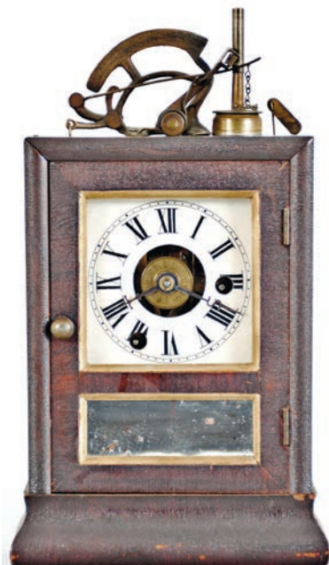
Circa 1860 Connecticut cottage clocks are everywhere, but not ones like this, and an Internet bidder paid $3540 (est. $700/900) to prove it. This Seth Thomas features an alarm that strikes a match and lights the top-mounted lamp at the selected time. Unrecorded is the number of homes incinerated when this malfunctioned. Polymath artist and inventor Rufus Porter patented the same idea in 1833; an exhibit devoted to Porter opens in December at the Bowdoin College Museum of Art in Brunswick, Maine.
