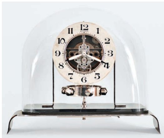
Atmos clocks by famed Swiss watchmaker Jaeger LeCoultre still are made and sold, but not ones like this circa 1935 predecessor. Jean Leon Reutter developed the concept of a "perpetual" clock that would not need winding, and this early model demonstrates the concept. Mercury and ammonia in a glass tube do the work using temperature changes. The mercury and ammonia, along with its oval glass dome, present serious shipping challenges. The high bidder, who we hope carefully hand-carried it home, paid $11,800, slightly under the $12,000/16,000 estimate.
