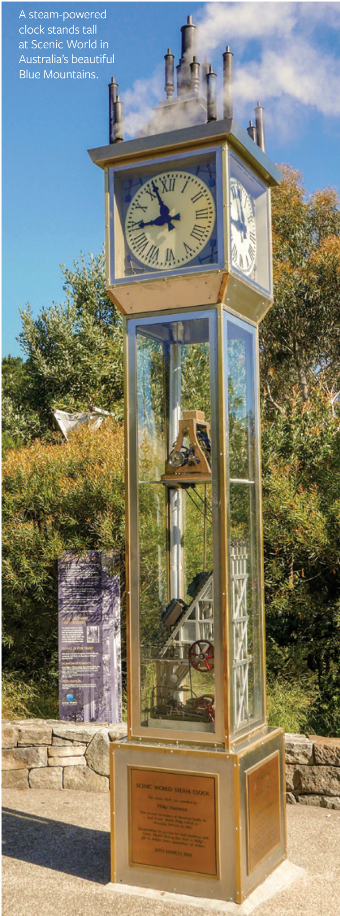
The steam clock's pinwheel escapement tops the movement made in Vancouver.
