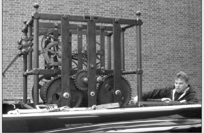
Figure 3. Philadelphia clock restorer John B. Spencer Jr. prepares the movement for unloading outside the Living History Center. The count and escape wheels are visible as is the unique central shift lever, which allowed both trains to be wound from a single arbor.
