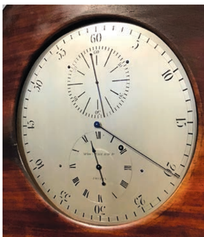
Astronomical regulators featured a special dial since the minutes and seconds were far more crucial than the hours for timing celestial observations. This dial adorns the third known example of Simon Jr.’s astros, on view in the Putnam Gallery of Harvard University’s Collection of Historical Scientific Instruments. Frishman photo.
