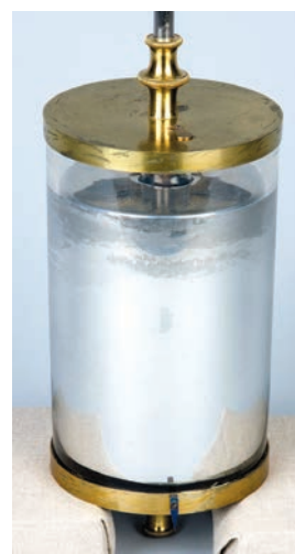
Many pounds of dense liquid mercury are visible in this glass-jar pendulum hanging in Simon Willard Jr.’s regulator clock at Harvard University. Mercurial pendulums made a major contribution to 18th- and 19th-century timekeeping accuracy, correcting for temperature variations and keeping accuracy to within seconds a month or better. Unlike the movement, which has English origin, the pendulum most likely was a Willard creation. Photo courtesy Collection of Historical Scientific Instruments, Harvard University.
