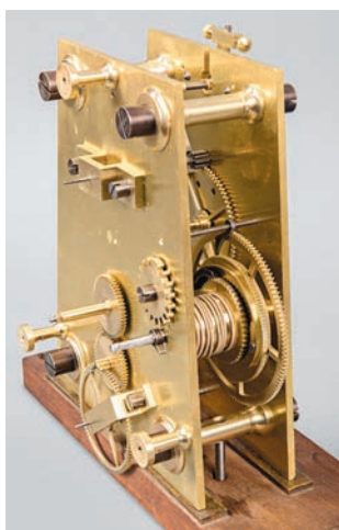
This finely finished high-precision time-only weight-driven eight-day movement occupies the top of the Willard House column-form floor clock. Nearly certain is that it was made in England for Simon Jr. to sell here. The case may have accompanied it from overseas, or more likely it was made here by a skilled joiner.
