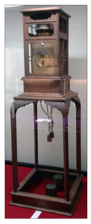
**Figure 7, left.** Early weight-driven Japanese clock with foliot escapement.
